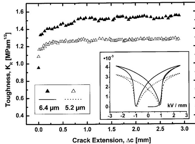
Fig. 2.  $R$ -curves for two different grain sizes with poling direction  $B$  along with the strain hysteresis for grain sizes of 5.2 and 6.4  $\mu\text{m}$ .
