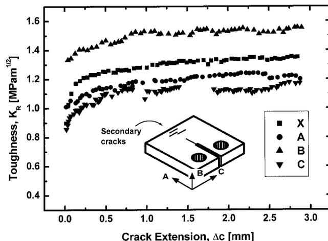
Fig. 1. R-curves for specimens with three different poling directions as contrasted to an unpoled specimen. The secondary cracks formed for the A-type specimens are indicated.
