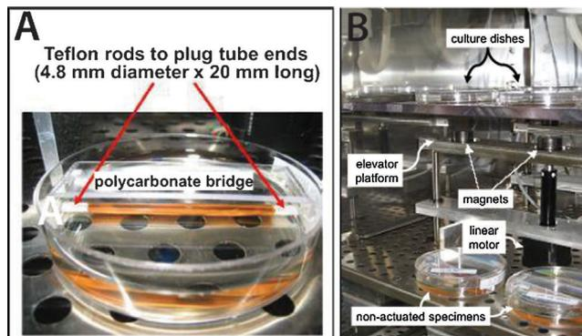
**Figure 2.** A: Wound cell-seeded tubular scaffold (6 cm long, eight wound fibril layers) in a culture dish. B: Computer-controlled magnetic elevators in cell culture incubator.
