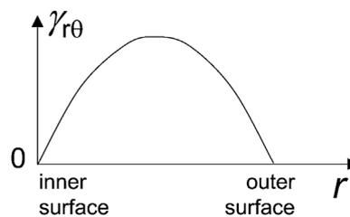
**Figure 4.** Functional form of shear strain variation through thickness of tube wall is quadratic.
