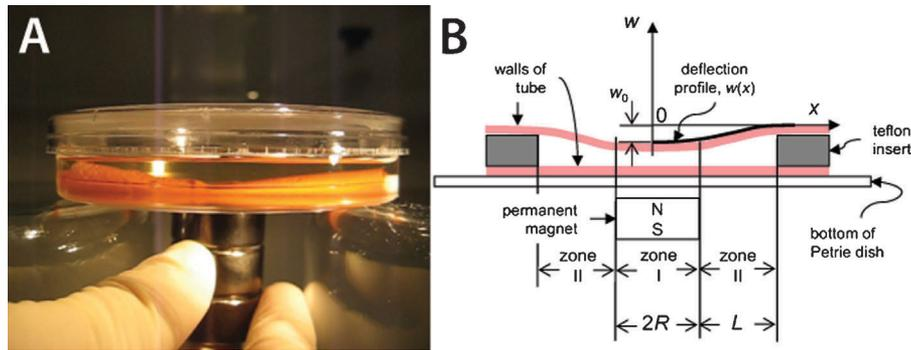
**Figure 3.** **A:** Wound tube scaffold deflecting down towards the bottom of the culture dish when approached from below by a hand-held permanent magnet. **B:** Schematic of different zones of deflection.
