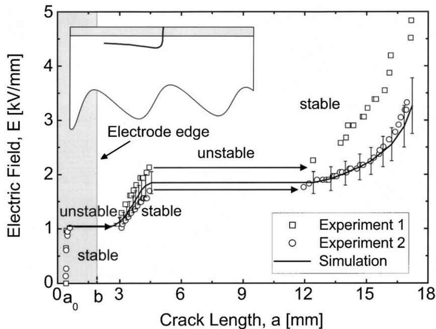
Fig. 6. Measured crack length as a function of the electrical field for the unpoled specimen with  $b=2$  mm. Note the four transitions between stable and unstable crack propagation. The crack path as observed in the optical microscope is shown in the insert.
