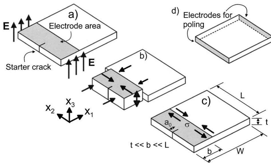
Fig. 1. Stress generation by mechanical clamping due to partial electrode coverage. (a) Electric field is applied at the electrodes (active material). (b) Shrinkage in  $x_1$  and  $x_2$  directions and expansion in  $x_3$  direction of the active part would ensue if the active part would be free. (c) Adjacent material mechanically clamps the active strip and high tensile stresses arise. (d) Electrode configuration for in plane poling.
