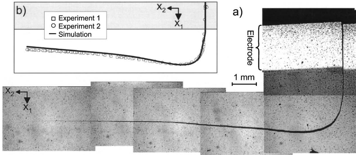
Fig. 5. (a) Photograph of final crack configuration for a curved crack in an unpoled specimen (b) Comparison of two different experiments and the simulation.<sup>11</sup>
